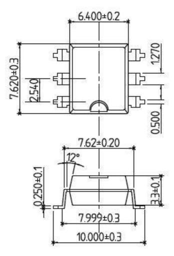
Note: No tolerance is marked as  $\pm 0.05$ mm.
