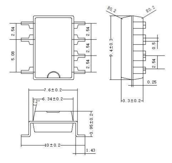
Note: No tolerance is marked as  $\pm 0.05$ mm.
