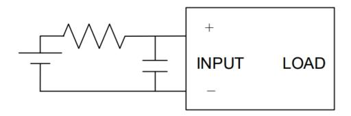
D. Recommended to use the circuit, the output peak voltage may cause SSR misoperation, so please add R/C circuit or varistor to absorb the peak voltage at the output end, see the following figure:
