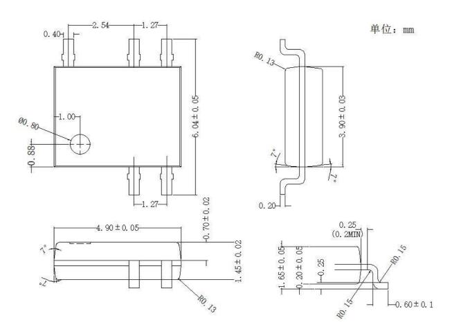
Note: No tolerance is marked as  $\pm 0.05$ mm.
