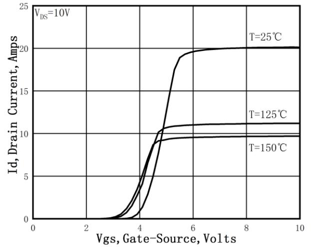
Figure 2. Transfer Characteristics
