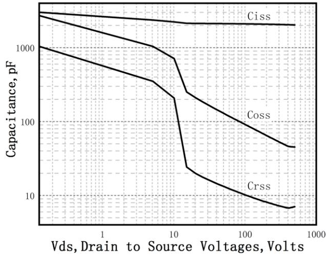
Figure 7. Capacitance Characteristics
