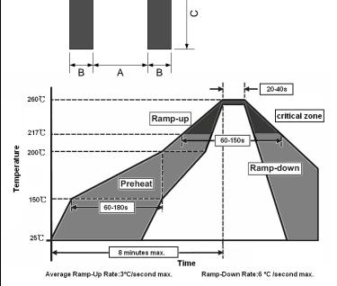
\* Recommended reflow methods: IR, Vapor phase, hot air \* Devices can be cleaned using standard industry methods
