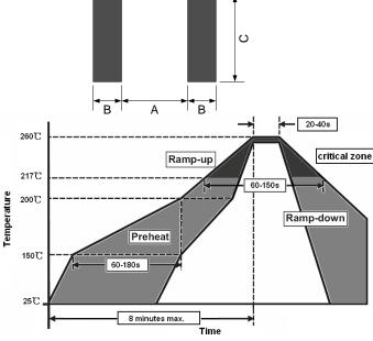
Average Ramp-Up Rate:3°C/second max. Ramp-Down Rate: 6 °C /second max. Package Information
